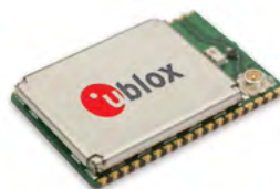
The ODIN-W160 multiradio module is ready-to-embed in industrial, medical and demanding IoT applications.
