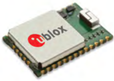
CAM-M8 series 9.6 x 14.0 x 1.95 mm
