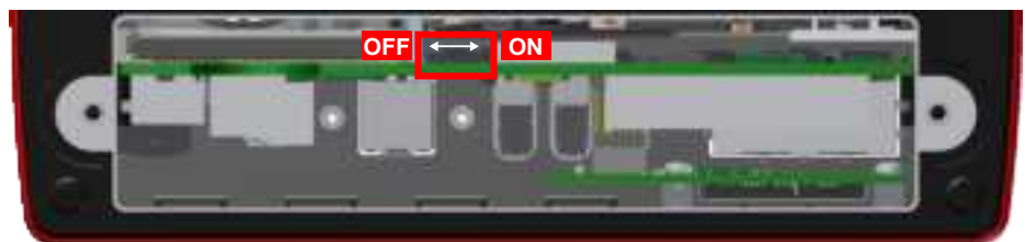
Figure 15: Power up/down switch in VN8914
