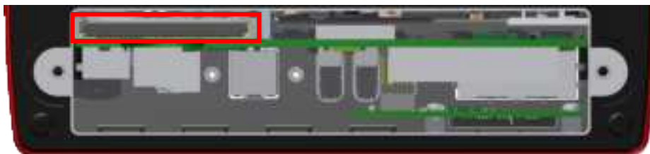
Figure 16: CFast card slot in VN8914
