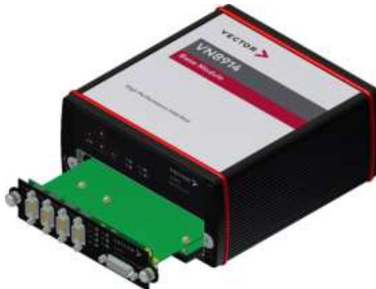
Figure 3: VN8914 with inserted VN8972 FlexRay/CAN/LIN Module
