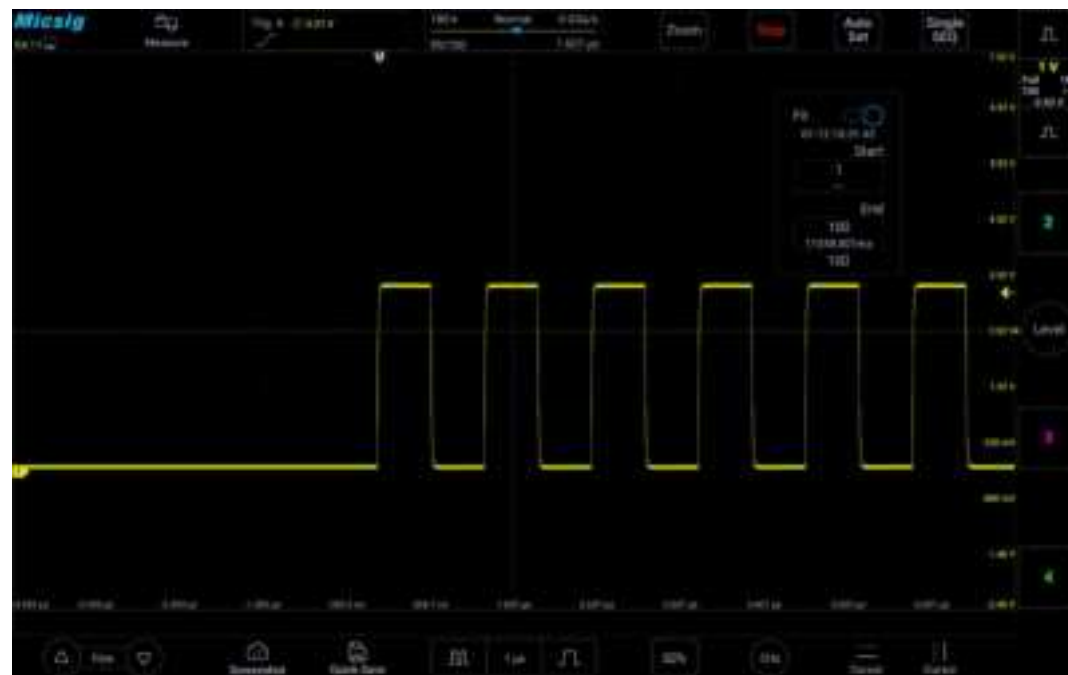
Figure 11-13 Segmented storage fitting view
