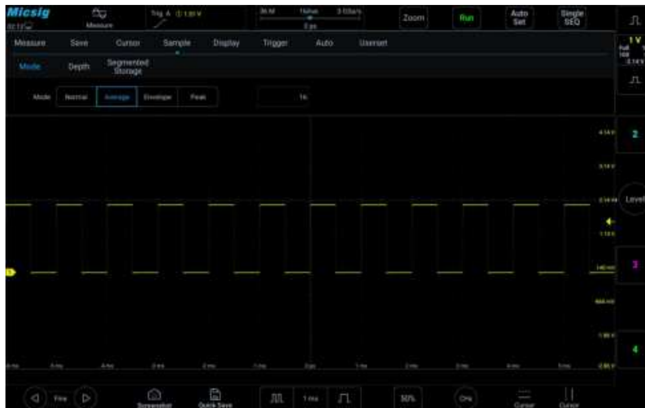
Figure 11-5 The waveform after selecting the average sampling mode, with the average number being 16.
