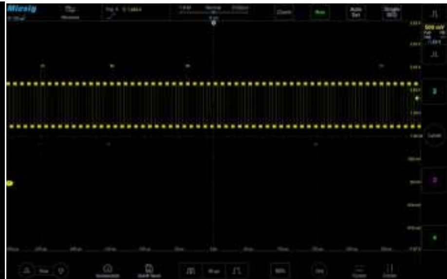
Figure 6-4 Abnormal Signal Captured by Setting Trigger Level
