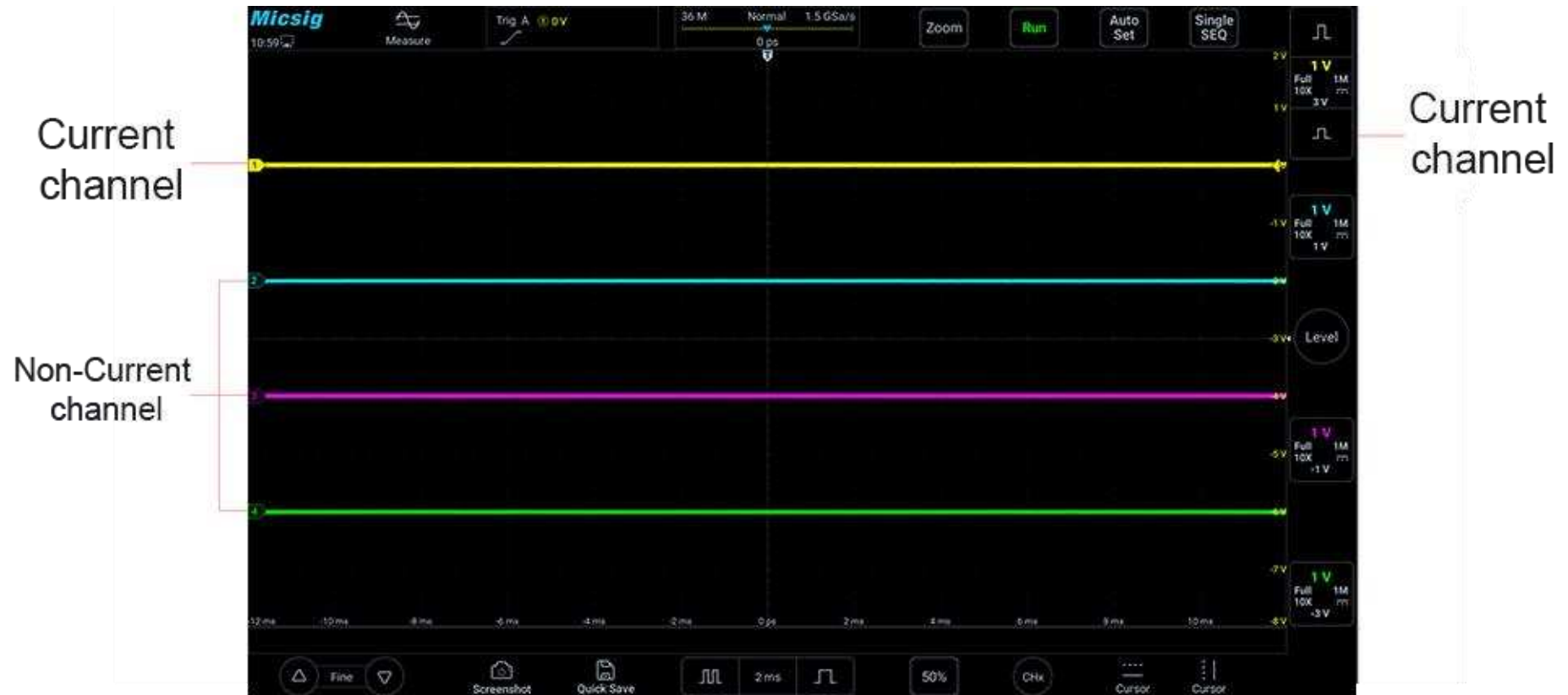
Figure 5-2 Current Channel and Non-Current Channel
