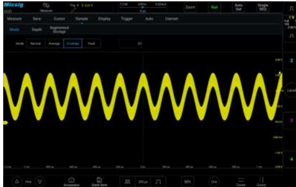
Figure 11-8 The amplitude modulation signal under the envelope sampling mode (32)
