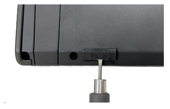
Figure 7-37 Opening the Fuse Protection Cover
