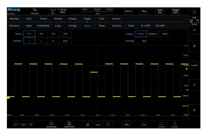
Figure 6-25 Runt Trigger Setting Menu
