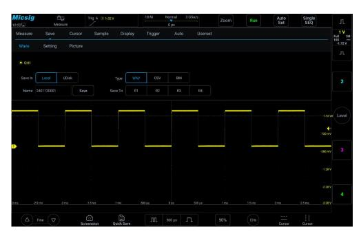
Figure 8-5 Save CH1 Reference Waveform Interface
