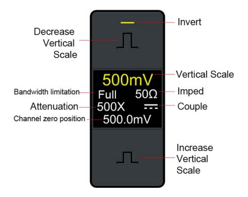
Figure 5-3 Channel Display Interface
