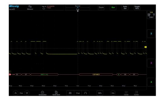
Figure 12-16 CAN bus decode interface
