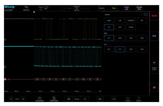
Figure 12-22 I<sup>2</sup>C Bus Configuration Menu
