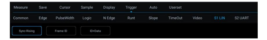
Figure 12-11 LIN Trigger Mode Configuration Menu
