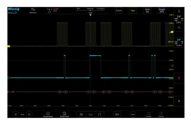
Figure 12-20 SPI bus decode interface
