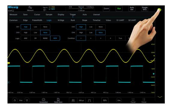
Figure 6-22 Trigger Level Adjustment
