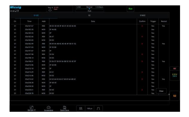
Figure 12-25 I<sup>2</sup>C Text Interface
