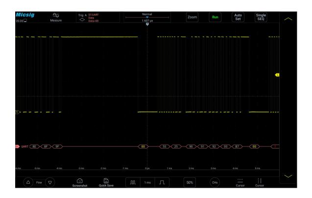
Figure 12-7 UART Decode Level Adjustment
