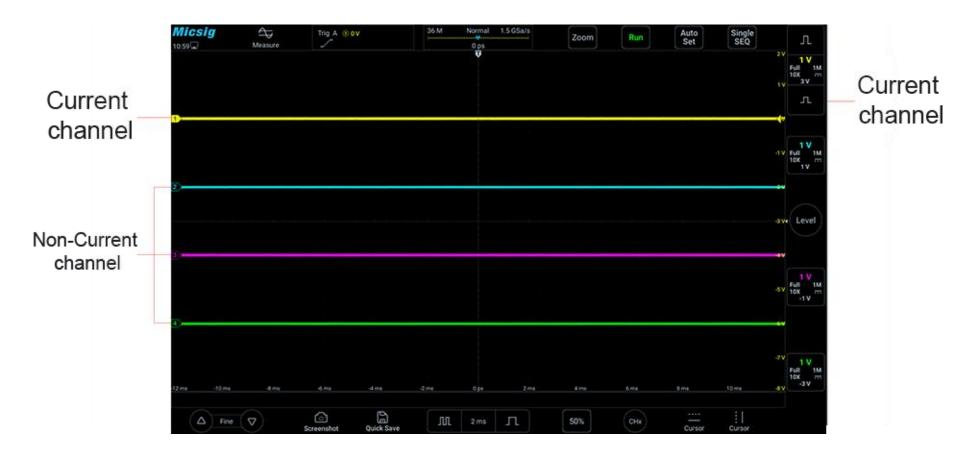
Figure 5-2 Current Channel and Non-Current Channel
