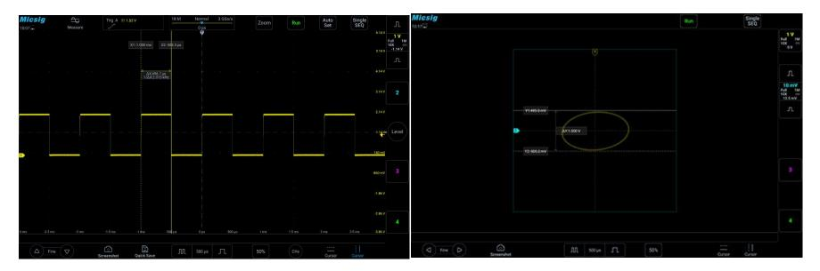
Figure 7-18 Cursor Measurement Pulse Width
