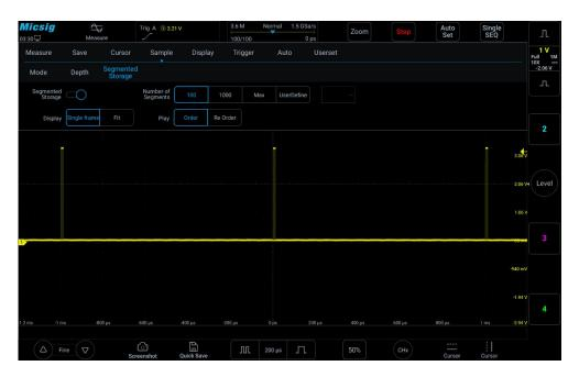
Figure 11-11 Segmented storage waveform acquisition
