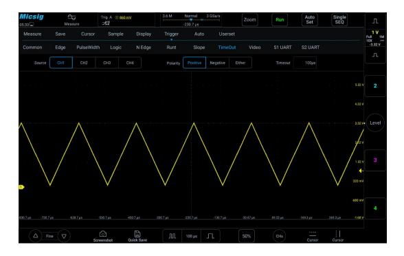
Figure 6-29 Time-out Trigger
