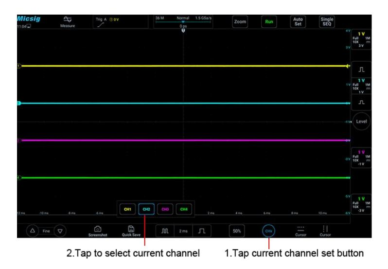
Figure 5-5 Using the Current Channel Selection Button
