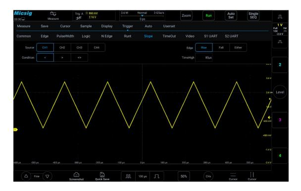
Figure 6-27 Slope Trigger Setting Menu
