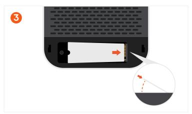
Insert the SSD at a slight angle (35-45°) and ensure it is fully seated in the PCle slot.
