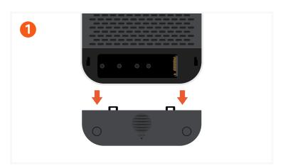
Remove the SSD enclosure cover on the bottom of the stand.
