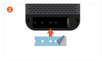
Before installing NVMe SSD, first apply the included thermal tape.
