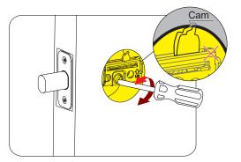
If the Latch bolt is stuck, remove the Latch bolt and chisel out a small channel at the top of the hole to give the Cam room to rotate.
