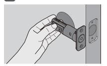
Hold the Latch in front of the door hole, flush the Latch against the door edge. Is the slot hole centred in the door hole?
