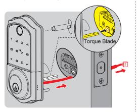
Install the Mounting Plate with the Mounting Plate Screws.
