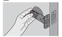
Hold the Latch in front of the door hole, flush the Latch against the door edge. Is the slot hole centred in the door hole?
