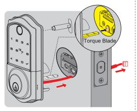
3 Install the Mounting Plate with the Mounting Plate Screws.
