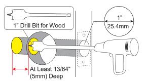
Extend the Latch hole at least 13/64" (5mm) deep by using a 1" (25.4mm) Drill Bit.
