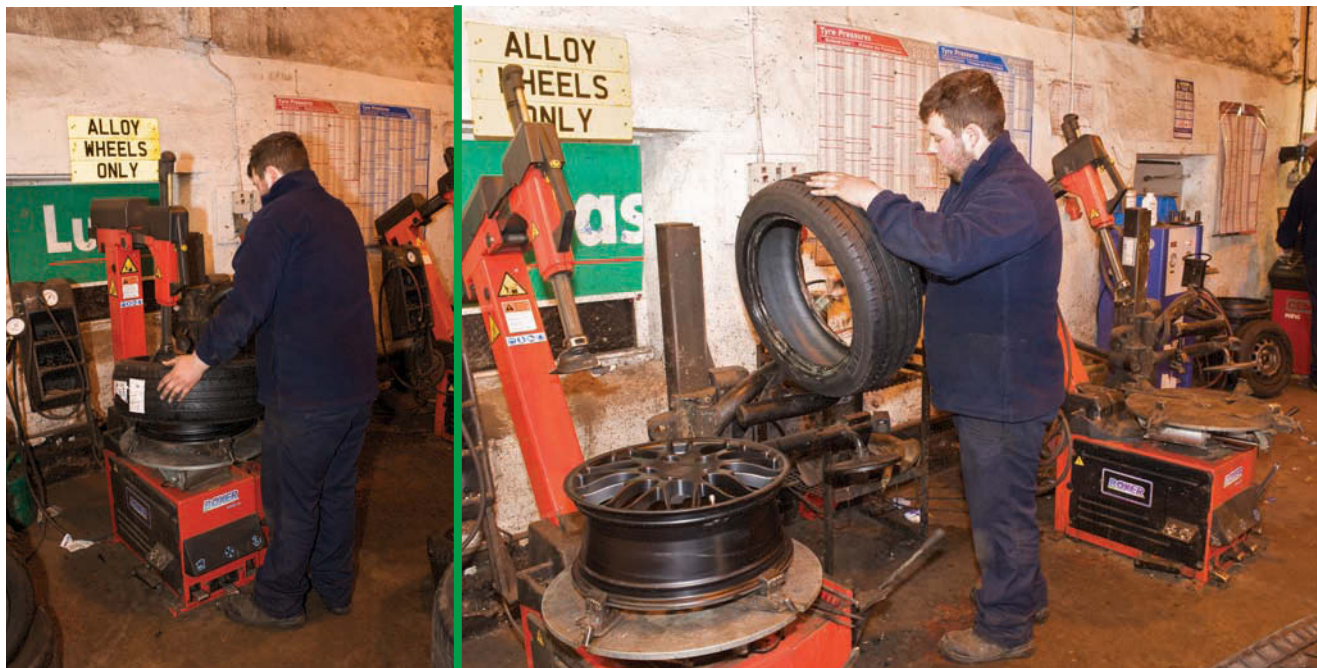
Honda and Fast Ford enthusiast, Nathan, gets on with winding tyres on to rims
