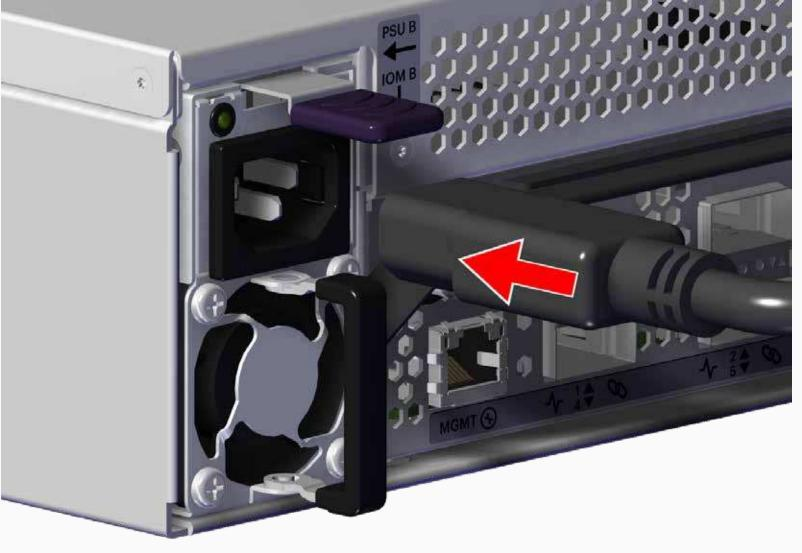
The enclosure has two power supply connections; install both power cords. The power range for
