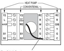
For 24VAC primary power, connect common side of transformer to "C" terminal.
