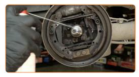
16 Install the new wheel hub with a bearing.
