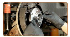
Tighten the hub. Use 12-point socket No.30. Use a torque wrench. Tighten it to 175 nm torque.
