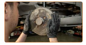
Tigten the brake drum fasteners. Use Torx T30. Use a torque wrench. Tighten it to 4 Nm torque.
