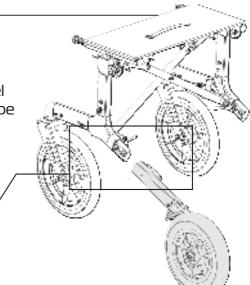
3. Depress the pin to allow the wheel to slide fully over the frame.
