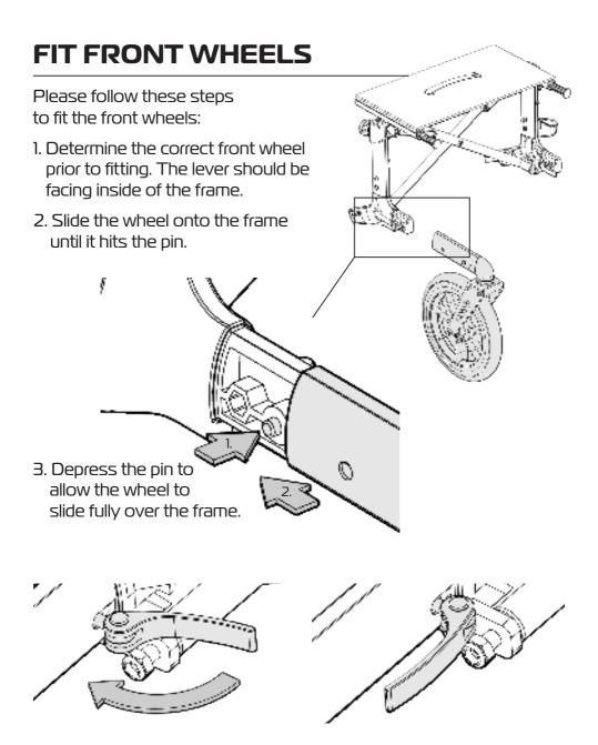
4. Flip the lever on the inside of the frame until tight to secure in place.
