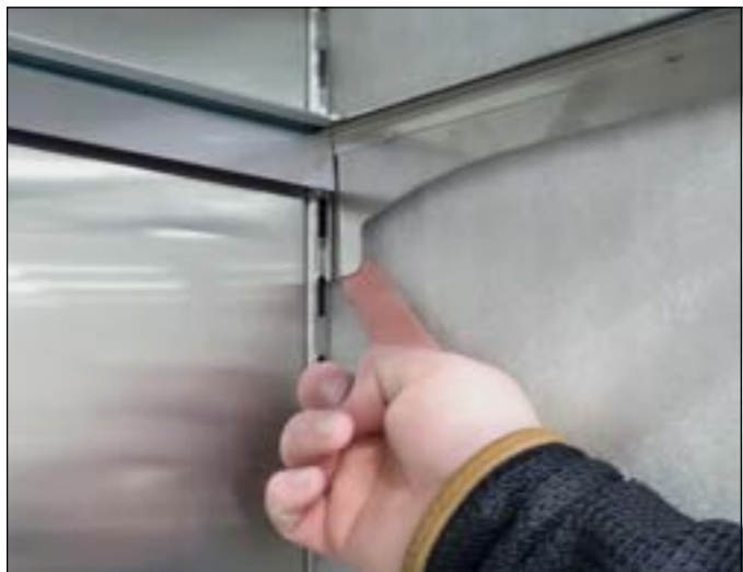
FIG. 6. Push the bottom tab inward.
