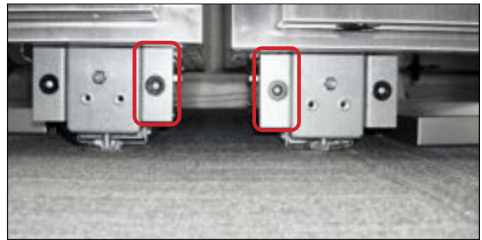
FIG. 11. Remove and discard the interior magnet brackets.
