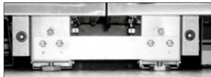
FIG. 18. Installed joining bracket.
