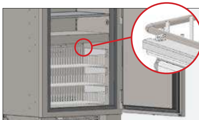
FIG. 3. Be sure the drawer sits under the rear tabs
