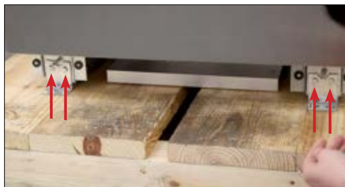
FIG. 7. Shipping bracket bolt locations.
