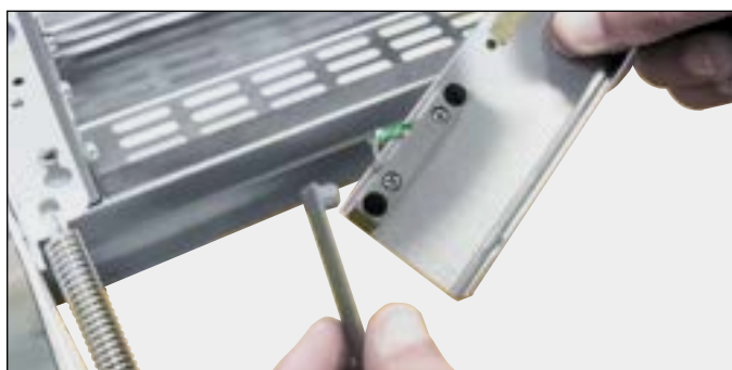
FIG. 4. Remove the plastic cover.
