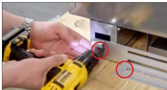
FIG. 8. Anti-tip bracket shipping bolt locations. Other side not shown.
