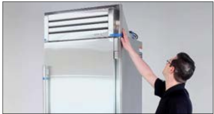
FIG. 2. Inspect the unit's exterior for visible damage.
