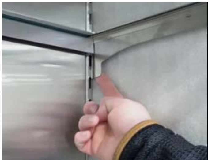
FIG. 6. Push the bottom tab inward.
