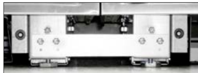
FIG. 18. Installed joining bracket.
