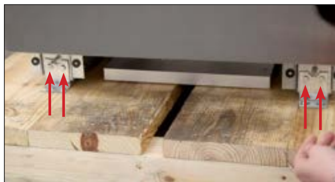
FIG. 7. Shipping bracket bolt locations.
