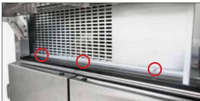
FIG. 9. Rainshield screw locations.
