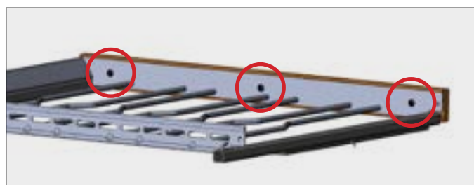
FIG. 2. Wine rack handle screw locations.
