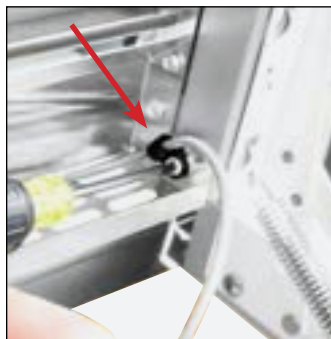
FIG. 6. Remove the p-clip holding the wire to the rainshield.
