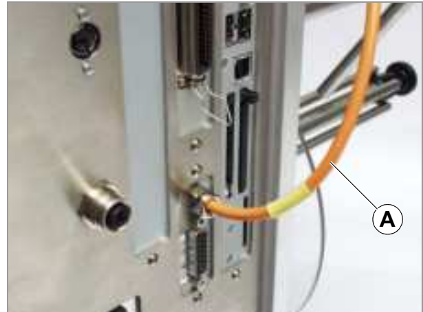
[18] OD sensor cable (A), internally connected to the USI.
