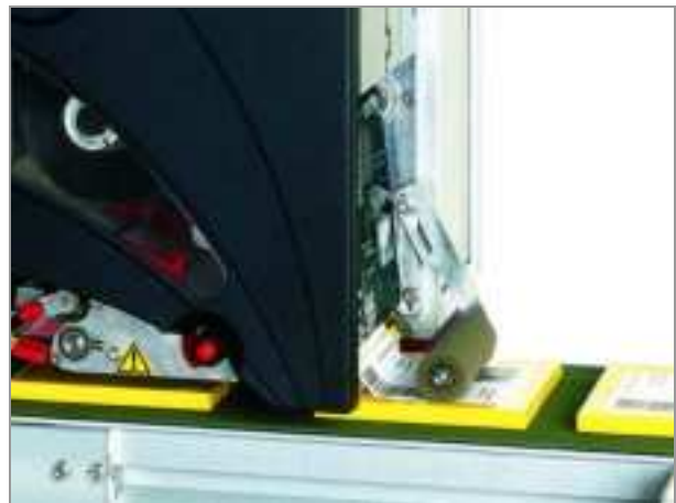
[4] Application example of the pressure roller.
