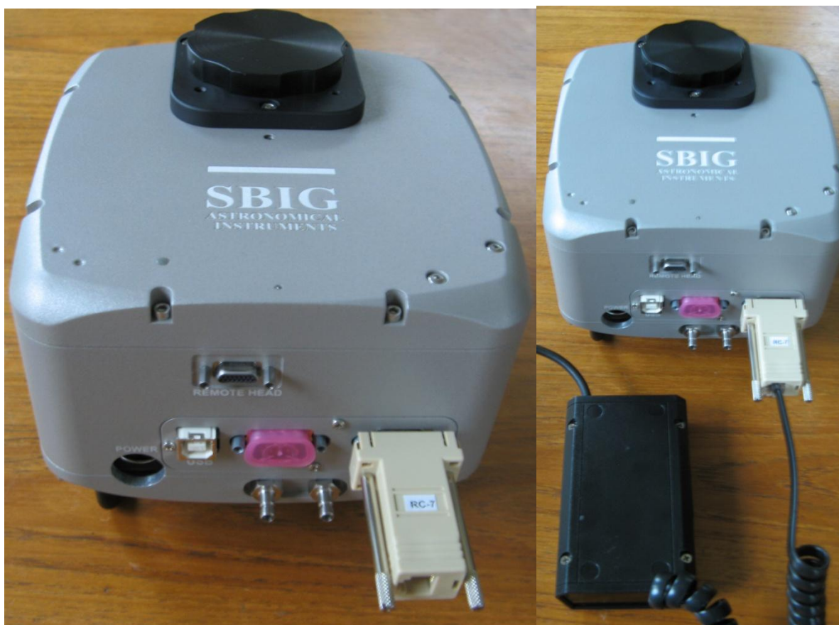
Figure 19A (left) The author's SBIG STL 11000M CCD camera with the adapter plug (labeled RC-7) plugged into the camera's autoguider output port. The female modular jack for an RJ-11 cable can be seen on the opposite end of the adapter, between the two metal set screws.
