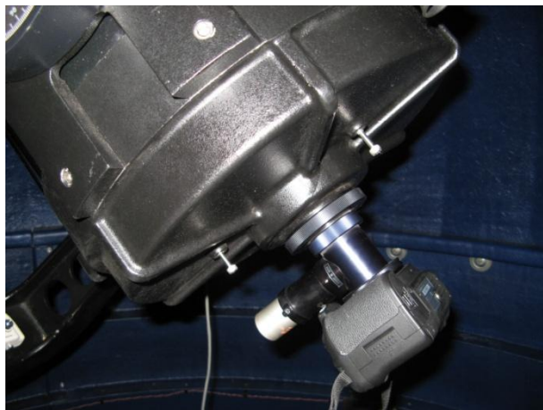
Figure 3. Off-axis guider and DSLR attached to the author's Compustar 14. This is a classic example of an uncomfortable position of a standard illuminated cross hair guiding reticle eyepiece in an off-axis guider. Imagine positioning yourself beneath the eyepiece to guide a long exposure astrophotograph.
