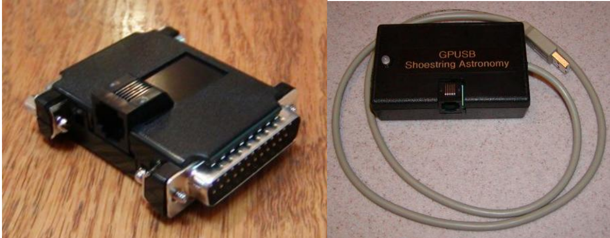
Figure 6A (left). A GPINT connector, available from Shoestring Astronomy. Note the male plug to be connected to the parallel port on the autoguiding computer and the female RJ-11 modular jack port with copper connection pins, where the RJ-11 cable can be attached.
