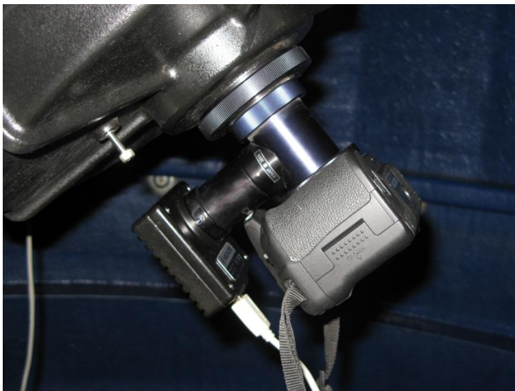
Figure 20. The Meade DSI serving as an autoguider camera in an off-axis guider in the same awkward, uncomfortable position shown in Figure 3. The autoguider can perform competently and tirelessly in this position, as long as required.
