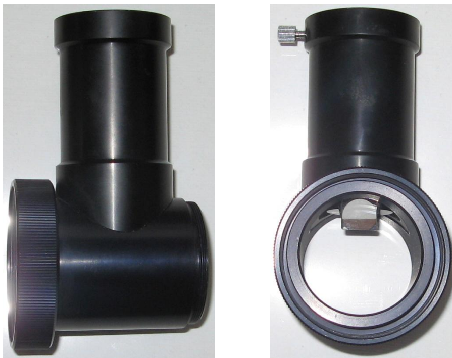
Figure 2A (left). An off-axis guider is a T-shaped connector that connects to the threads of the rear cell of the Compustar with the threaded ring at left. The threads to the right accept a T-ring for a camera or other adapter. The vertical “stem” of the T accepts an illuminated cross hair reticle eyepiece with which the precise position of the guide star and guide errors can be judged.
