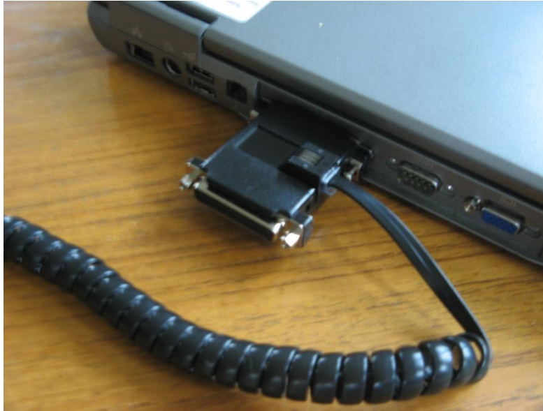
Figure 7. The GPINT connector attached to the parallel port of the autoguiding computer and a coiled RJ-11 cable inserted into its female modular jack plug.
