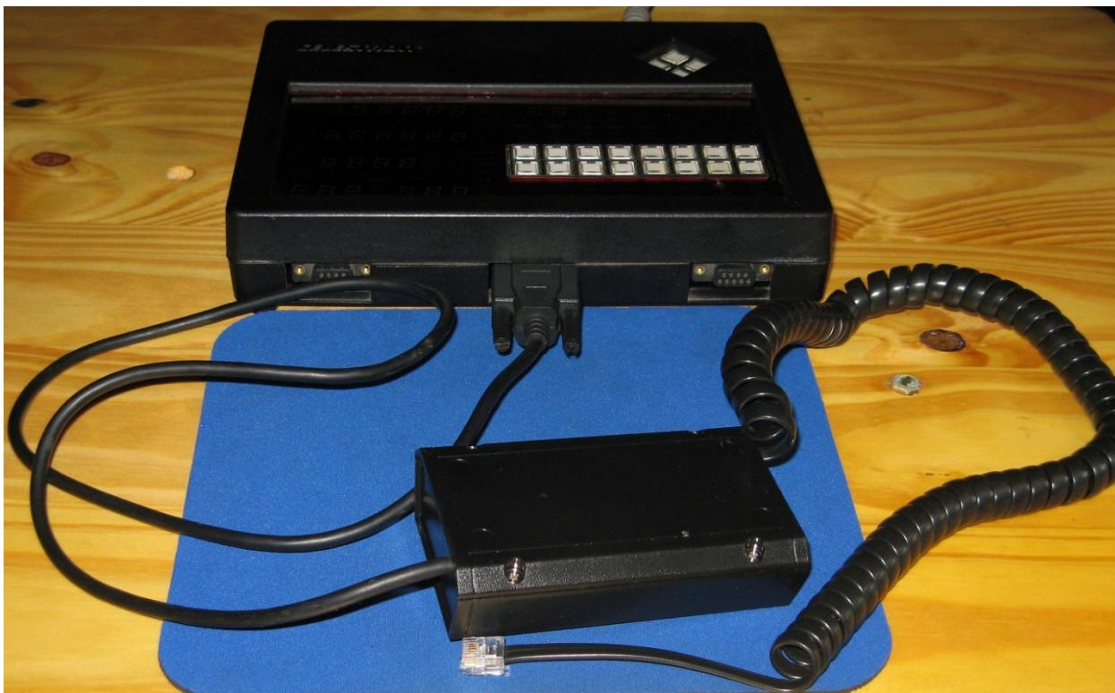
Figure 16. The assembled autoguider relay box. The coiled RJ-11 input cable with its modular jack at bottom center is not connected to the autoguiding computer in this illustration (see Figure 7 for illustration of that connection). The male DB-9 connector is plugged into the central port on the Compustar computer module. The computer module is not powered up in this illustration.
