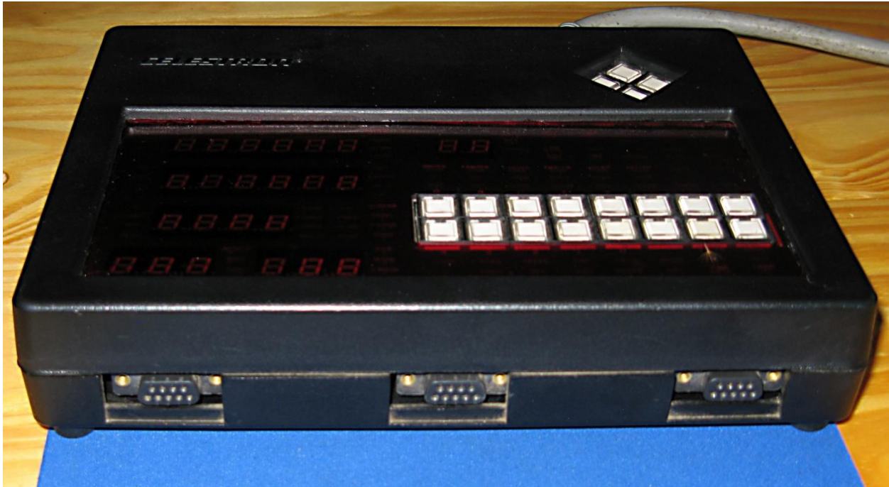
Figure 9. The front edge of the Compustar computer module showing its three female DB-9 ports. Each port receives 9 pins. The right port is for an optional joystick, the left port is for output to a printer. The center DB-9 port is the guide port for autoguiding input.
