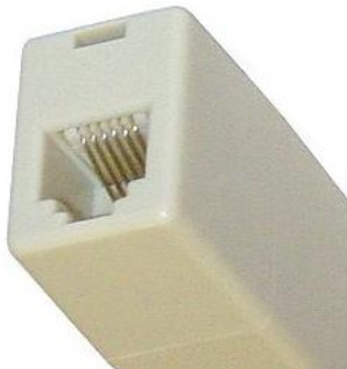
Figure 8. A female RJ-11 modular jack guide port, with copper connection pins, on a modern telescope mount. One simply inserts the jack on the opposite end of the RJ-11 cable into this guide port to complete the link between the autoguiding computer and the telescope mount to enable autoguiding. However, the Compustars don't have such a guide port.
