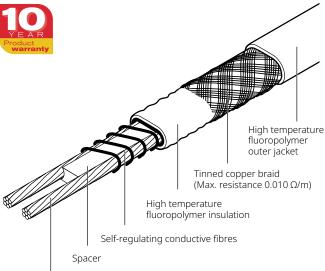
2.3 mm<sup>2</sup> nickel plated copper conductors
