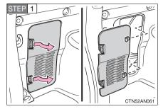
Disengage the claws and remove the cover.
