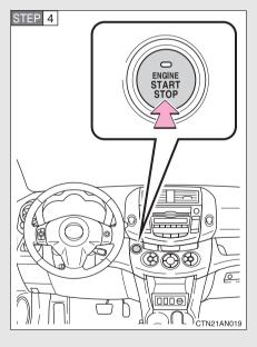
Press the "ENGINE START STOP" switch.
