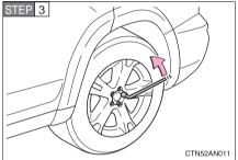
Slightly loosen the wheel nuts (one turn).
