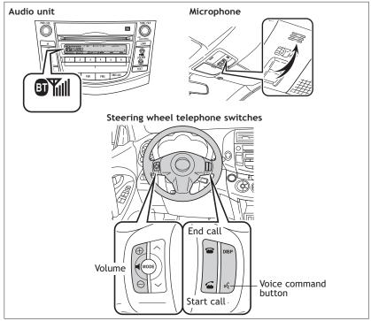
Bluetooth® technology allows dialing or receipt of calls without taking hands from the steering wheel or using a cable to connect the compatible telephone and the system.
