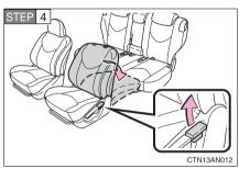
Pull the seatback angle adjustment lever up to unlock and push down the seatback.
