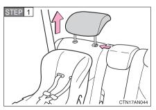
Remove the head restraint.
