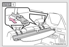
Attach the hooks to the head restraints.
