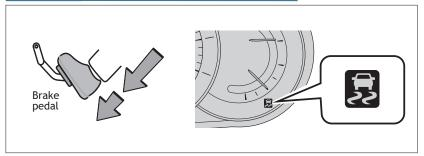
HAC helps prevent rolling backwards on an incline. To engage, push further down on brake pedal while at a complete stop until a beep sounds and slip indicator illuminates. HAC holds for approximately 2 seconds after releasing brake pedal.
