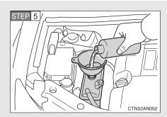
Add engine coolant if necessary.
