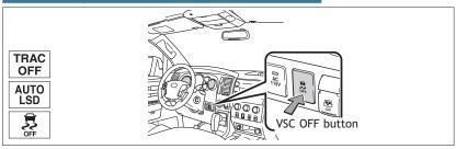
The VSC OFF button is used to switch between modes related to the TRAC, VSC and Auto LSD functions (2WD models.)
