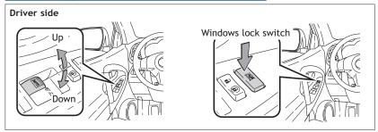
Automatic operation (driver side only) Push the switch completely down or pull it completely up and release to fully open or close. To stop window midway, lightly push the switch in the opposite direction.
