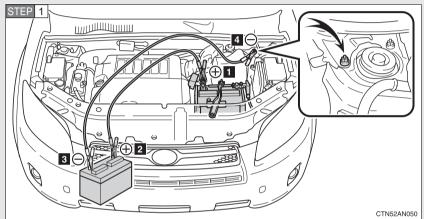
Connecting the jumper cables
