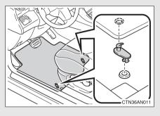
Secure the driver's floor mat using the hooks provided.
