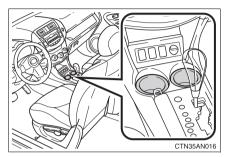
Removing the adapters changes the size.  $(\rightarrow P. 308)$
