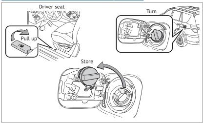
**NOTE:** Tighten until one click is heard. If the cap is not tightened enough, Check Engine " $\stackrel{\Box}{\bowtie}$ " indicator may illuminate.
