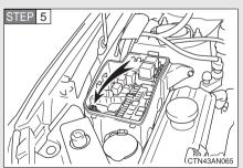
Remove the fuse with the pullout tool.
