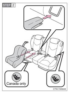
Latch the buckles onto the LATCH anchors.
