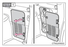
Disengage the claws and remove the cover.
