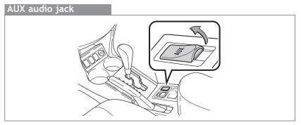
By inserting a mini plug into the AUX audio jack, you can listen to music from a portable audio device through the vehicle's speaker system while in AUX mode.
