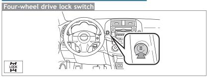
Push the switch to ensure that the engine torque is applied to the four wheels.
