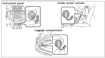
**NOTE:** Designed for car accessories. Engine switch/"ENGINE START STOP" switch must be in the "ACC" or "ON" position to be used.
