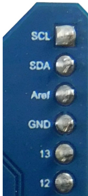
Figure 3. CN2 connector for I 2 C/I 3 C connection
