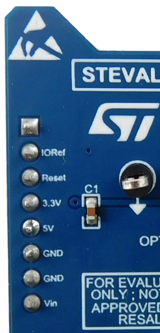
Figure 2. CN1 connector for 3.3V power supply
