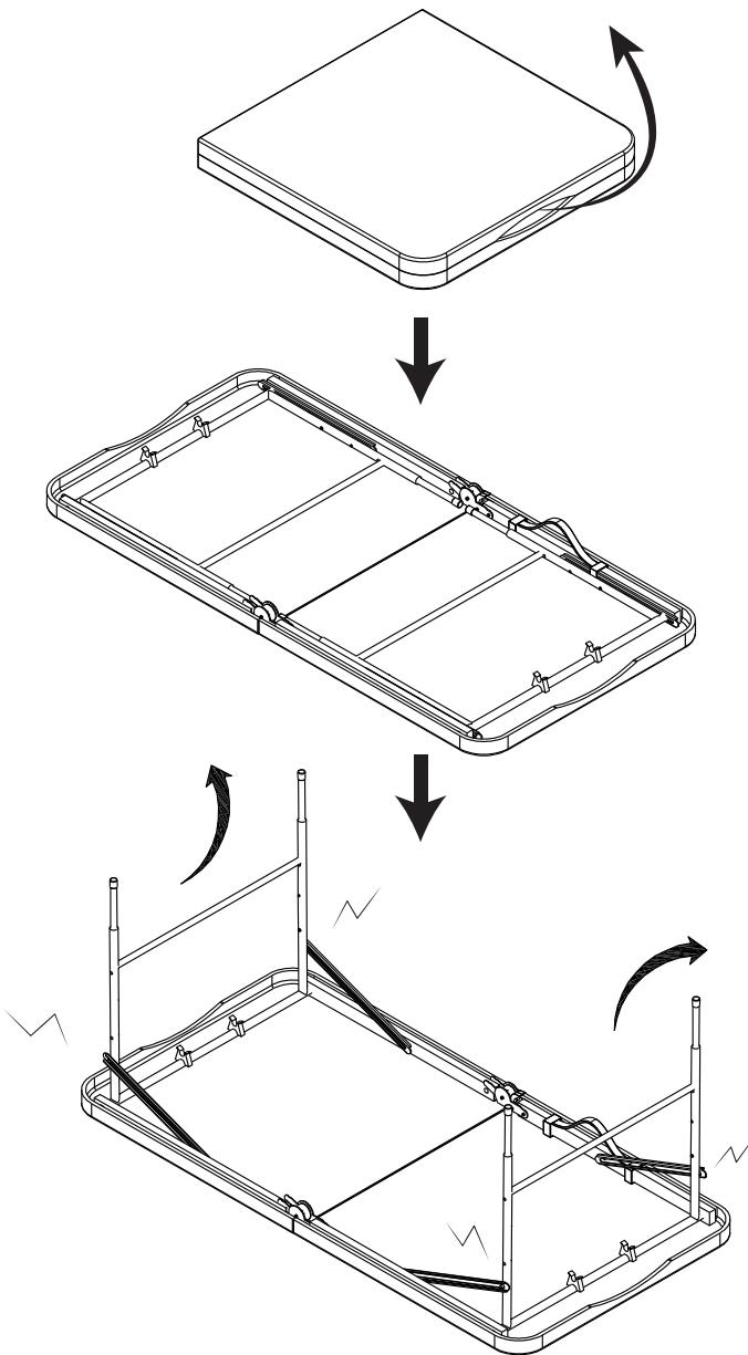
**EN:** 2. Adjust the table leg. First press the spring button on one side and press it into the tube, then pull out the table leg a little so that the spring button no longer pops out, and then press the spring button on the other side to pull out the table leg.
