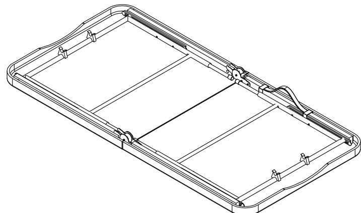
**EN:** 3. Pull the side lock trigger and fold the table at the same time, placing the handle outside the table.
