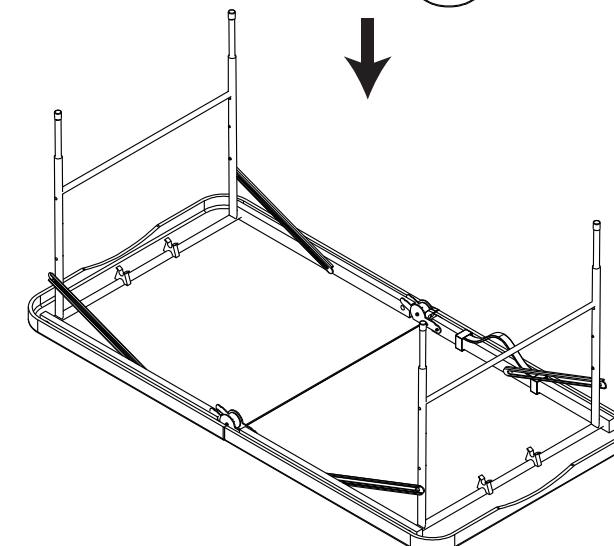
**EN:** 2. Press the support poles on both sides to unlock the table legs and fold them.
