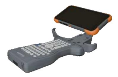
2. Press down and snap the other edge of the Archer 4 under the locking clip.
