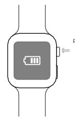
Press and hold for 3 seconds to turn the watch on or off.
