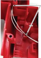
Place the white NTC wires into wire traps as shown.
