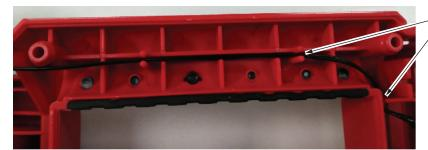
Place the black NTC wires into wire traps as shown.
