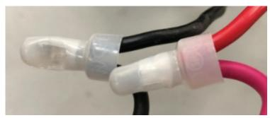
Crimp motor black wire and PCB black wire together using close end connector. Crimp motor red wire and PCB red wire together using close end connector.
