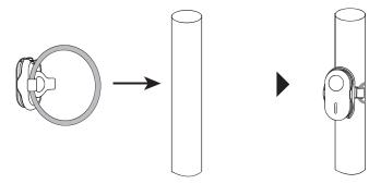
The Mini Remote can rotate freely when attached to the Mini Remote Strap.
