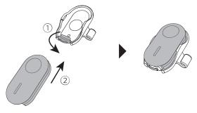
Choose an appropriate Mini Remote Strap and hook it onto one side of the Mini Remote Base. Wrap it around any mounts or accessories, such as a selfie stick, then hook it onto the other side of the base.
