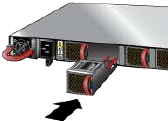
Figure E-3: Inserting Fan Module
