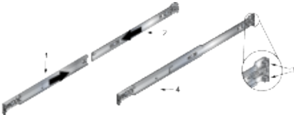
1 Rail-slide 2 Rail-rod 3 Rack plugs (detail) 4 Rail (assembled)
