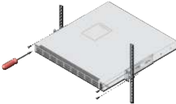
Figure 3-4: Inserting the Switch into the Rack
