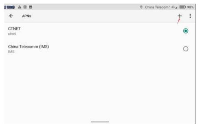
4. Check the setting information for different mobile operators, then save after the configuration. The "Name" and "APN" is required, while the others depend on the specific situation.
