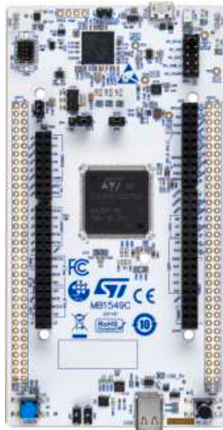
Figure 1. STM32U5 Nucleo-144 board
