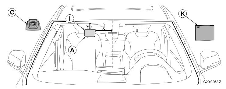
The front camera with display **C** must not restrict the driver's view. The front camera with display **C** must be installed within the windscreen wiper's wipe area and outside the coloured sun protection strip (screen printed strip).
