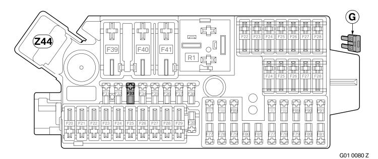
Insert fuse **G** into slot **F33** in power distributor **Z44**.
