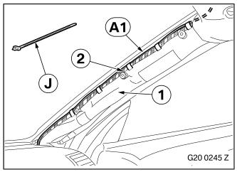
Secure branch **A1** to the standard wiring harness (2) with cable ties **J** so as not to adversely affect the function of the airbag (1). ◀
