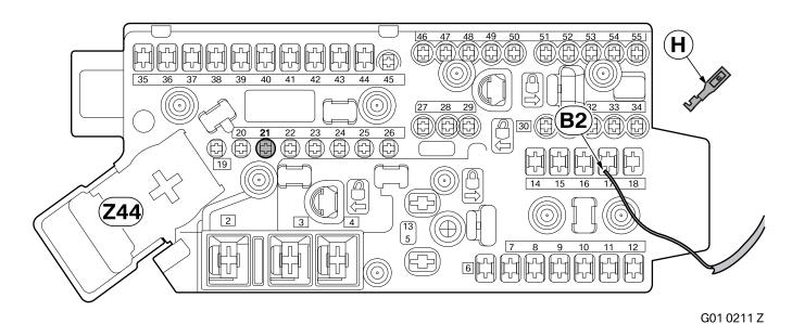
Connect branch B2, RED cable, as follows to power distributor Z44:
