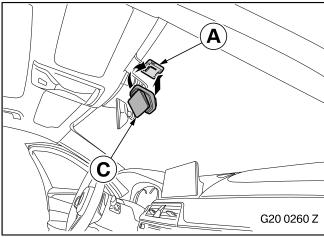
Fit front camera with display  ${\bf C}$  as shown in the base  ${\bf A}$ .
