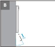
Use **torx wrench** to screw **M3x7.5 Torx head screw** into the screw hole on the bottom of device diagonally upward.
