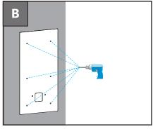
Use a **6mm electric drill** to make six holes with 25mm depth in the screw holes of wall-mounting template.
