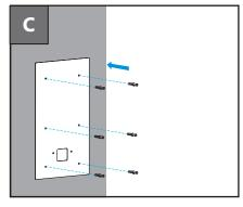
Insert six plastic wall anchors into the holes.
