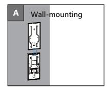
Hang the device onto the square hanger on the wall-mounting box.
