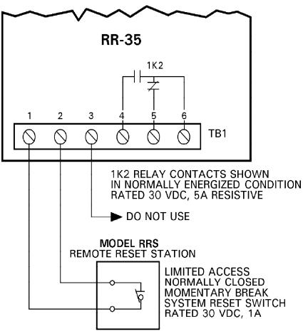
SUPERVISED, POWER LIMITED REMOTE RESET STATION CONNECTIONS RATED 24 VDC, 100mA MAX TOTAL CONNECTION RUN LINE RESISTANCE 3 OHMS MAX
