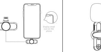
Step 2:Press switch button of microphone,the indicator will turn to green ,and then the power is turn on.
