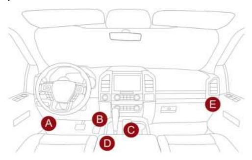
Usually, the OBD port is located under the dashboard, above the pedal on the driver's side. The five locations shown lite the picture are common OBDII port locations.
