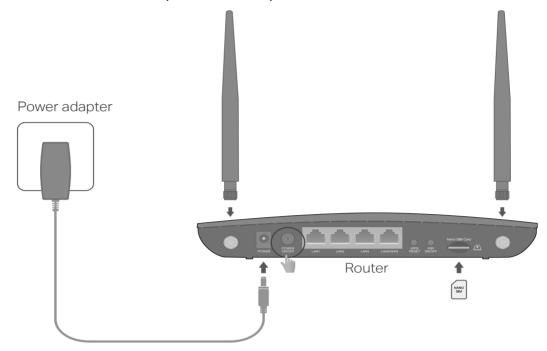
2. With the gold contacts facing down, insert the Nano SIM card into the slot until you hear a click.
