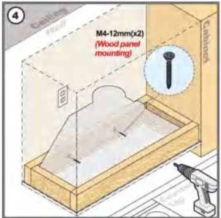
(4) Through the installation holes, fasten the range hood using woodscrews to mount onto the wood blocking.
