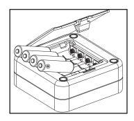
Flip open hatch on backside of Alarm Unit, insert 4x AA batteries (not included) into Alarm Unit, ① side of battery facing away from springs. Close hatch.
