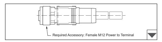
Female M12 connector for power terminal not included. Insert connector into Detection Unit end labeled "power", taking note of locating feature on connector for proper alignment. Twist until locked. Connect end of cable to machine/system power.
