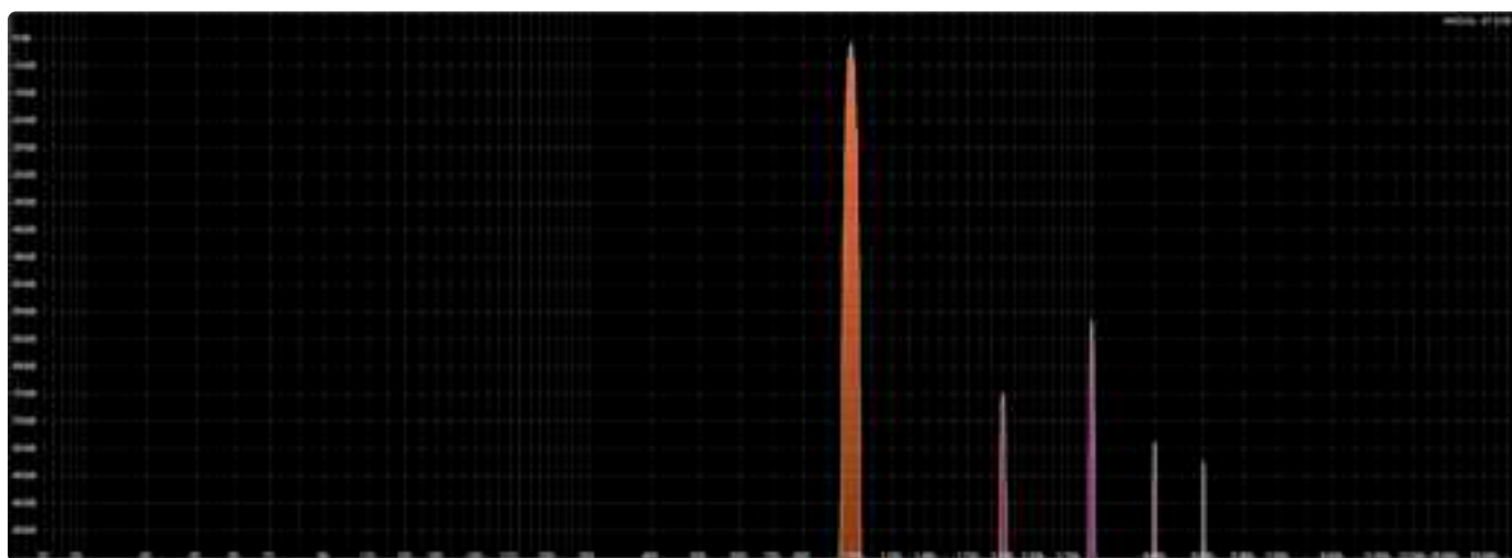
Example of additional harmonics generated using a 1kHz tone. ('High' Density)
