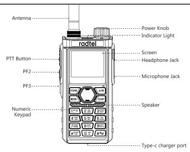
PF2 Button: Short press to turn on FM RADIO, long press to switch High/Middle/Low power PF3 Button: Short press to SEEK frequency from nearby radio, long press to open squelch
