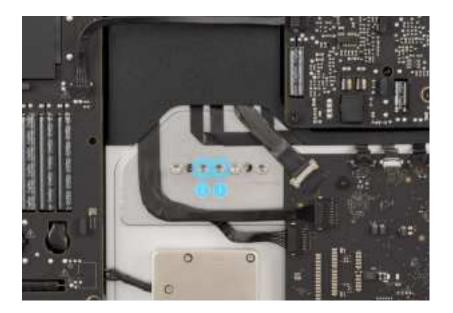
6. Use the adjustable torque wrench and 20IP bit to fully reinstall the right 20IP screw to 2.9 Nm.
