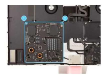
9. Install the 3 mm alignment pin in the upper left screw hole in the right side of the housing (1). Then install the 4 mm alignment pin in the upper right screw hole (2).
