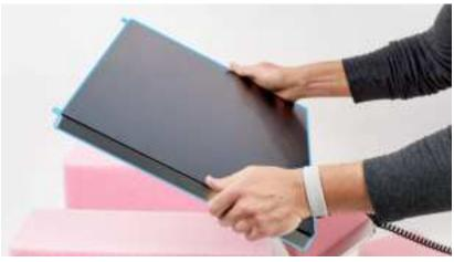
12. Separate the display just enough to remove the release liner from the bottom edge of the display. Repeat the motion along the perimeter of the display until the release liners are removed from the left, right, and top edges.
