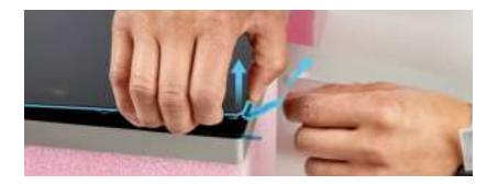
14. Remove the liner from the sticky sheet pad. Roll the silicone roller back and forth on the sticky sheet pad to clean it.
