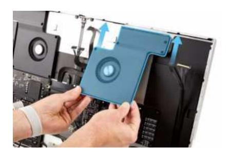
4. Position the top part of the fan next to the speaker. Then position the lower part of the fan into the housing.
