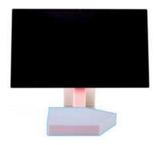
4. Place the support foam rest blocks perpendicular to the display with the lines in the blocks running vertical as shown.
