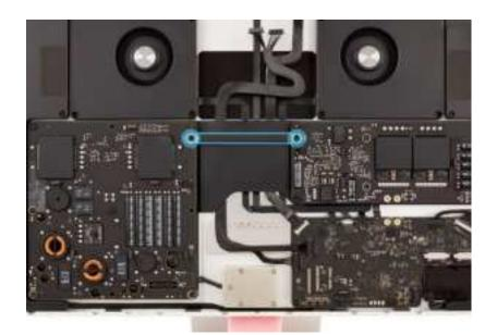
20. Position the logic board bus bar between the logic board and DC power supply board. Then use the T6 screwdriver to partially reinstall the four T6 screws (923-07141).
