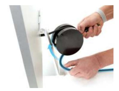
2. Hold the cord and the power cord removal tool with the same hand. Ensure that the cord is aligned with the port. Use your other hand to hold the stand for stability.
