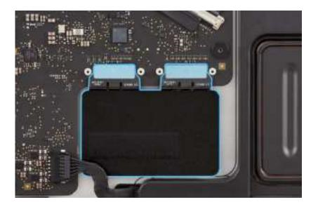
6. Position the two USB-C board connector cowlings over the ends of the two flex cables. Use the T3 screwdriver to reinstall the four T3 screws (923-05561).
