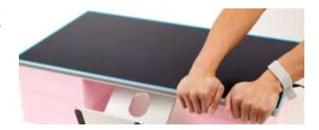
16. Place the display in the microfoam bag. Then place it flat on a clean table with the display side facedown. Wait 30 minutes for the adhesive to attach to both the display and the housing.
