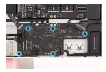
7. Use the black stick to move the cables out of the way as you lift the logic board out of the housing.
