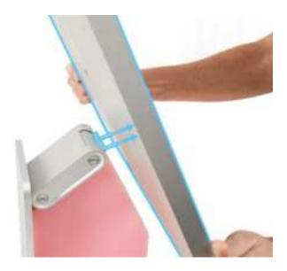
4. Remove the alignment pins from the stand.
