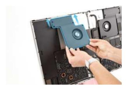
4. Position the top part of the fan next to the speaker. Then position the lower part of the fan into the housing.
