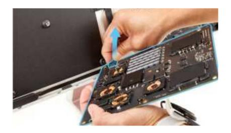
6. Remove the PFC power supply board from the housing and set it aside.
