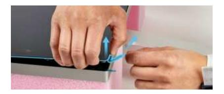
13. Remove the liner from the sticky sheet pad. Roll the silicone roller back and forth on the sticky sheet pad to clean it.
