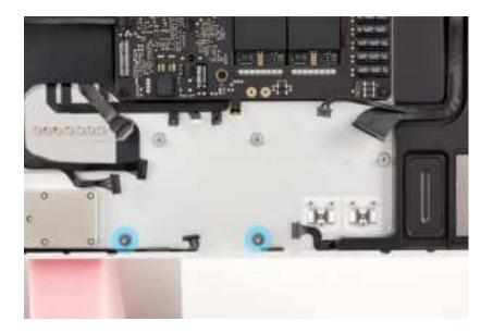
2. Use the two 2 mm alignment pins to position the logic board into the housing while using the black stick to move the cables out of the way.
