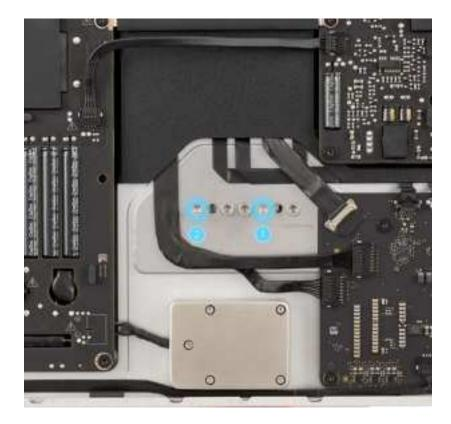
10. Keep the 20IP bit in the 2.5–25 Nm adjustable torque wrench. Set the torque value to 6.4 Nm. Use the adjustable torque wrench and 20IP bit to fully reinstall the four 20IP screws in the order shown.
