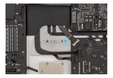
7. Remove the two alignment pins. Use the adjustable torque wrench and 20IP bit to partially reinstall two 20IP screws (452-07329) in place of the alignment pins in the order shown.
