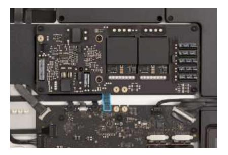
6. Starting with the DC power supply board on the right, use the T8 screwdriver to remove the six T8 screws (923-07143). Then remove the DC power supply board.
