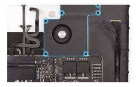
2. Use the black stick to gently release the adhesive between the fan flex cable and the housing as shown.
