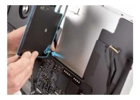
Use the black stick to flip down the locking lever on the fan flex cable. Reapply the adhesive cover. Then rotate the fan toward the housing.
