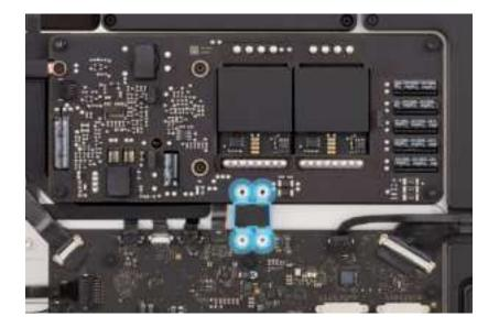
23. Slide the end of the power supply signal flex cable into the connector. Use the black stick to flip down the locking lever. Then press the polyester film tab to adhere it to the flex cable.
