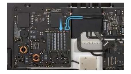
13. Position the power supply bus bar on the power supply boards. Then use the T6 screwdriver to partially reinstall the two T6 screws (923-07141) into the bus bar.
