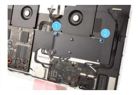
10. Turn over the DC power supply board to reinstall the original power supply signal flex cable. Slide the end of the flex cable into the connector. Use the flat end of the black stick to flip down the locking lever. Then press the polyester film tab to adhere it to the flex cable.
