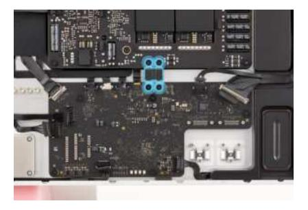
6. Use the T6 screwdriver to remove the five T6 screws (923-07142) from the logic board.
