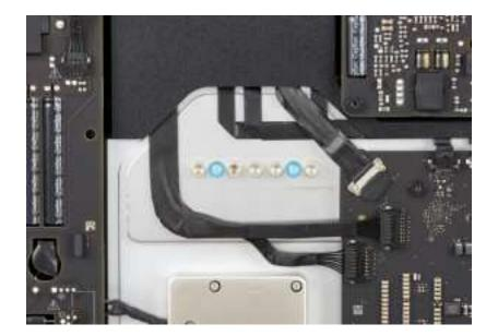
10. Keep the 20IP bit in the 2.5–25 Nm adjustable torque wrench. Set the torque value to 6.4 Nm. Use the adjustable torque wrench and 20IP bit to fully reinstall the six 20IP screws in the order shown.
