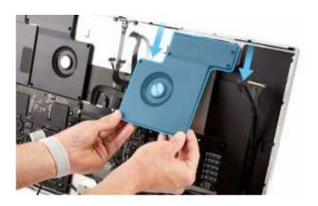
5. Rotate the fan to directly access to the fan flex cable connector.
