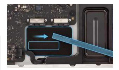
5. Press the ends of the two flex cables to the connectors.
