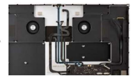
8. Run the flat end of the black stick along the length of the flex cable to adhere it to the housing.
