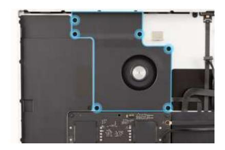
2. Use the black stick to gently release the adhesive between the fan flex cable and the housing as shown.
