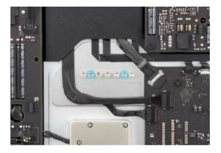
2. Replace the removed screws with the alignment pins for stand and VESA mount adapter.
