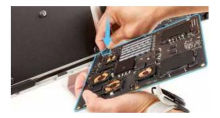
6. Align the upper left and upper right screw holes of the PFC power supply board over the two alignment pins.
