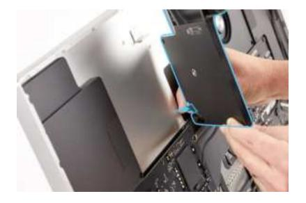
2. Use the black stick to flip down the locking lever on the fan flex cable. Reapply the adhesive cover. Then rotate the fan toward the housing.
