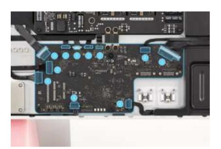
14. Slide the ends of the five cables into the connectors (4).
