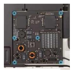
10. Use the black stick to lift the left side of the PFC power supply board from the housing. At the back of the board, pinch the levers at the end of the power cord port cable. Then slide the end of the cable out of the connector. Remove the PFC power supply board from the housing.
