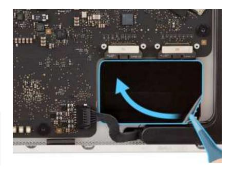
4. Use the T3 screwdriver to remove the six T3 screws (923-07144). Then use the black stick to remove the boards from the housing.
