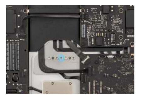
7. Use the adjustable torque wrench and 20IP bit to partially reinstall the remaining four 20IP screws to 3.5 Nm in the order shown.
