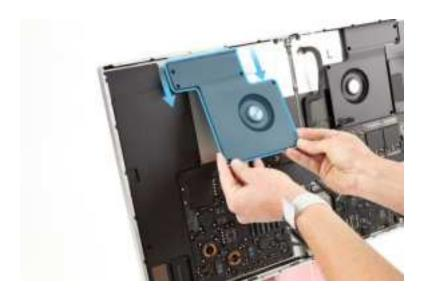
5. Rotate the fan to directly access to the fan flex cable connector.
