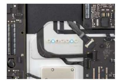
3. Use the adjustable torque wrench and 20IP bit to remove the middle 20IP screw (452-06710) and the four outer 20IP screws (452-06708) in the order shown.
