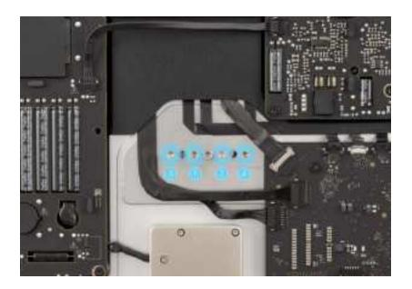
8. Remove the two alignment pins. Then use the adjustable torque wrench and 20IP bit to partially reinstall two 20IP screws (452-06708) as shown.
