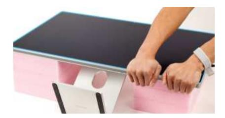
17. Place the display in the microfoam bag. Then place it flat on a clean table with the display side facedown. Wait 30 minutes for the adhesive to attach to both the display and the housing.
