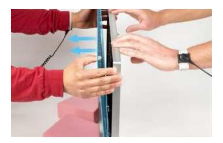
6. Carefully separate the remainder of the display from the housing. When the display is separated from the hangers in the housing, lift up the display assembly and rest it on the support lift wedge and support tilt wedge.
