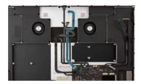
19. Use the black stick to position the cable cover over the cables in the middle of the housing. Then press along the edges of the cable cover to adhere it to the housing.
