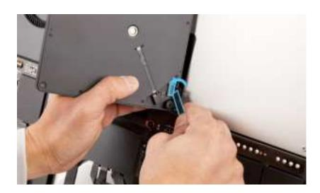
7. Slide the end of the fan flex cable out of the connector. Then remove the fan from the housing.
