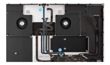
16. Use the black stick to peel the microphone flex cable from the housing to remove it.
