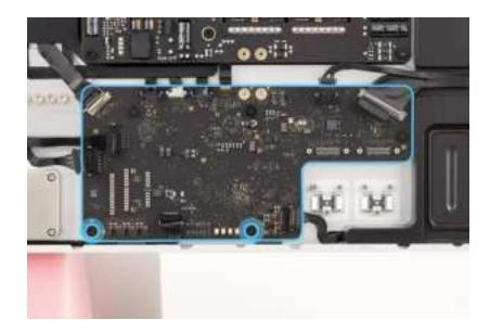
Position the logic board bus bar on the logic board and the power supply board. Use the T6 screwdriver to partially reinstall the four T6 screws (923-07141).
