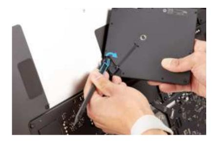
7. Slide the end of the fan flex cable out of the connector. Then remove the fan from the housing.
