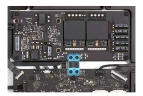
3. Pinch the sides of one end of the power supply signal cable and slide it out of the connector. Then repeat this step on the other end of the power supply signal cable.
