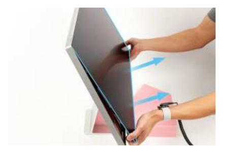
6. Carefully separate the display from the housing, ensuring that you clear the hangers near the top of the housing. Support the bottom of the display with one hand while you tilt the top of the display away from the housing.
