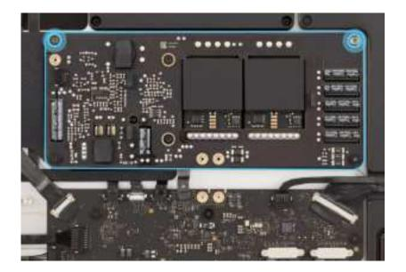
17. Position the power supply bus bar on the power supply boards. Then use the T6 screwdriver to partially reinstall the two T6 screws (923-07141) into the power supply bus bar.
