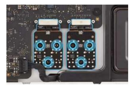
3. If you're replacing the USB-C boards, peel the polyester film tape from the adhesive backing. If you're reinstalling the existing USB-C boards, skip to reassembly step 4.
