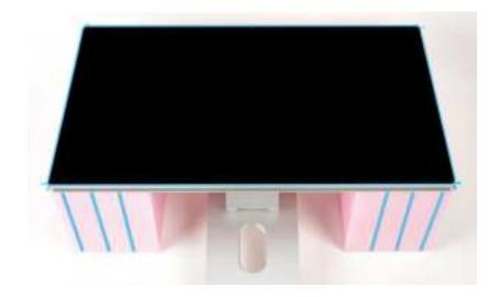
13. Separate the display just enough to remove the release liner from the bottom edge of the display. Repeat the motion along the perimeter of the display until the release liners are removed from the left, right, and top edges.
