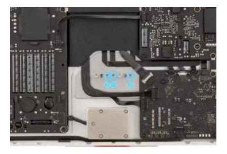
5. Set the torque value to 2.9 Nm. Use the adjustable torque wrench and 20IP bit to partially reinstall the two 20IP screws to 2.9 Nm in the order shown.
