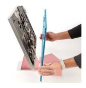
Position the support foam rest blocks under the housing as shown. Then place the display on the foam rest blocks in front of the housing.
