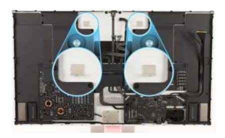
11. Place the two large foam blocks on the table with the lines in the blocks running vertical as shown. Place the entire unit on top of the foam blocks with the display faceup. Remove the support wedge. Then align the display with the housing.
