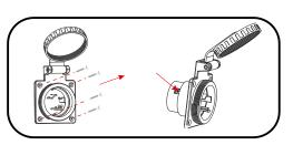
Turn off Rv's main breaker. Use a screwdriver to Test your new inlet for proper fit loosen and remove the four screws and pull out the old inlet out of the RV. Loosen screws and disconnect the old inlet to any wires.
