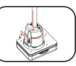
Install the rear housing and tighten the screw. (3.0-3.9 In/Lb).
