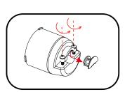
Loosen the screws and remove the cable bushing, this may be needed later.
