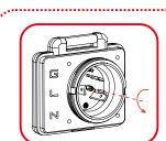
For Hipot Test-Make surethe screw is loose.
