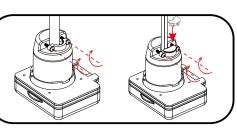
Tighten the screws on the strain relief clamp until they are snug around the cable. You may need to use the optional bushing to have a proper snug fit. (4.5-5.5 ln/Lb).
