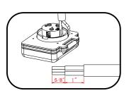
Please strip the wires as shown; strip off 1 5/8" of the outer insulation layer of the cable, and only 5/8" of the colored insulation of the conductor cables. Make sure the wire condition is good, full strands and shiny copper.
