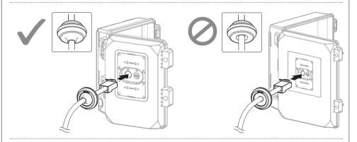
\* Ensure that the bushing is correctly installed inside the product.
