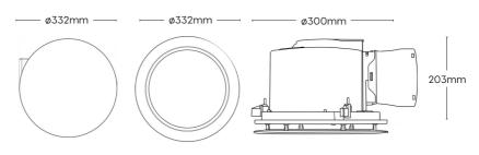
Ø300MM CUT-OUT SIZE Ø148MM DUCT SIZE
