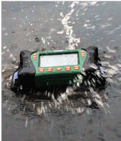
Drop-proof and Waterproof housing meets IP67 standards.
