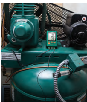
SD750 3-Channel Pressure Meter/Datalogger (p. 109)
