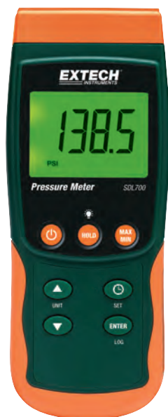
Optional Pressure Transducers available in: 30psi (PT30) 150psi (PT150) 300psi (PT300)
