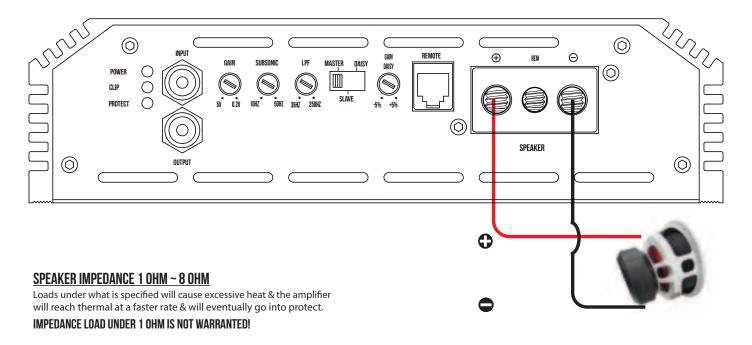
We recommend using minumum 8 Ga speaker cables to acquire the intended performance & efficiency. Run the speaker cables from your speakers to the amplifier's mounting location.
