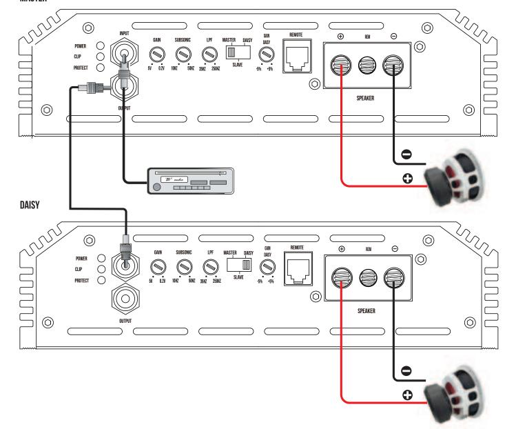
In daisy chain mode, the master amplifier's audio settings, such as gain, crossover, etc., are routed to the amplifier marked as daisy. From that daisy amplifier, you can route the input signal from the master amplifier to a second daisy by using the output RCA on the first daisy amplifier. You can continue adding amplifiers in a chain this way.
