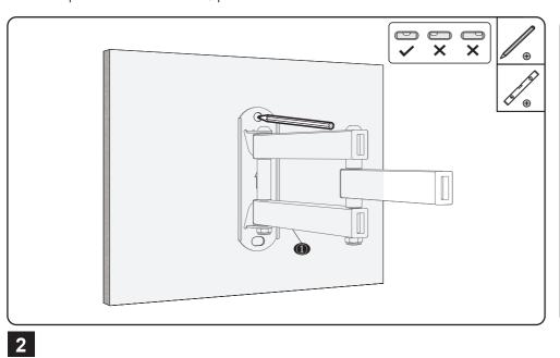
2 Drill 3/8" (10mm) diameter x 2.6" (65mm) length holes at the marked position.
