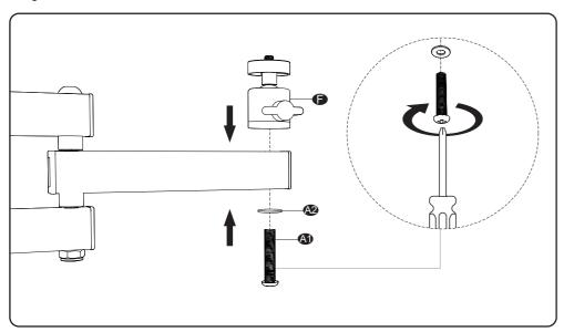
2.2 Adjust the desired angle and tighten the thumb screw
