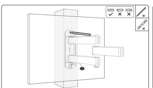
2 Drill 3/16" (4.5mm) diameter x 2.6" (65mm) length holes at the marked position.
