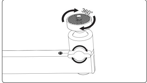
3.2b: No Screw Adapter Required Attach projector to the Spherical Universal Head •
