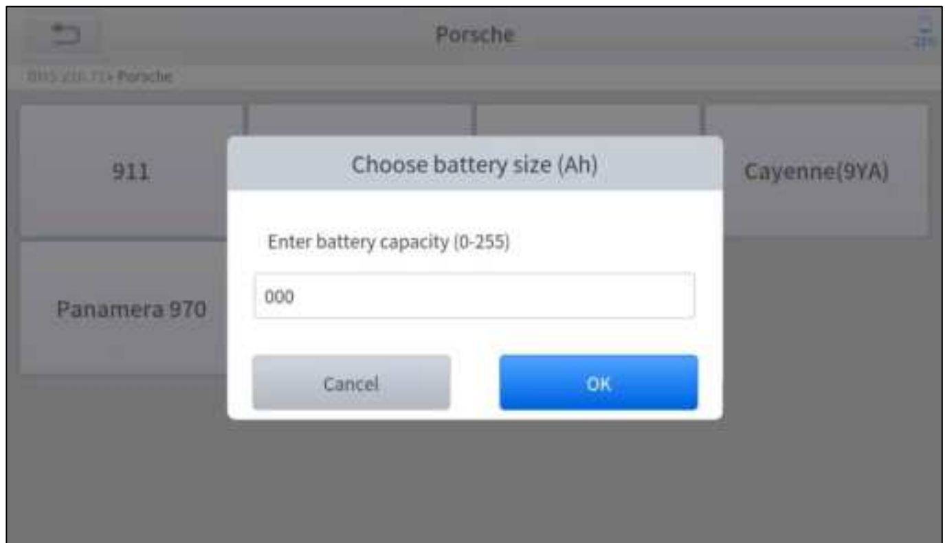
Figure 5-17 Sample of BMS function (screen 1)
