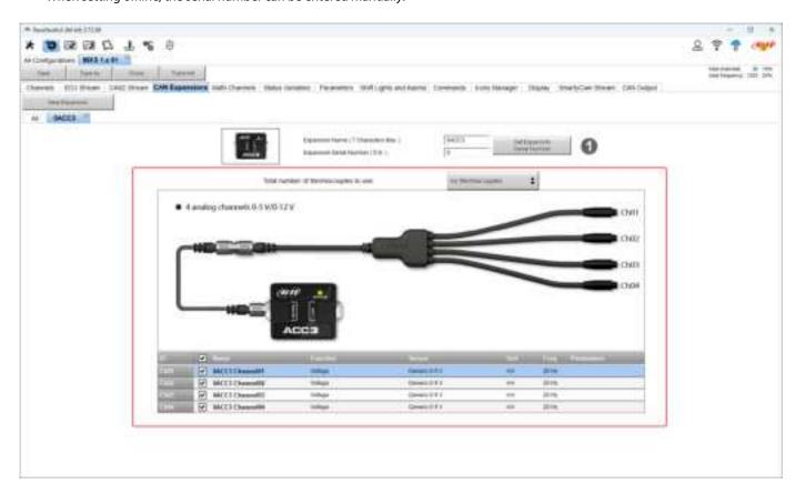
Select the cable in use, which strictly depends on the number of thermocouple sensors you plan to use. Make your selection in the **total number of thermocouples to use** (2 in the example).
