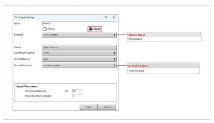
When the configuration is finished save and transmit it to the logger using the software top left keyboard.
