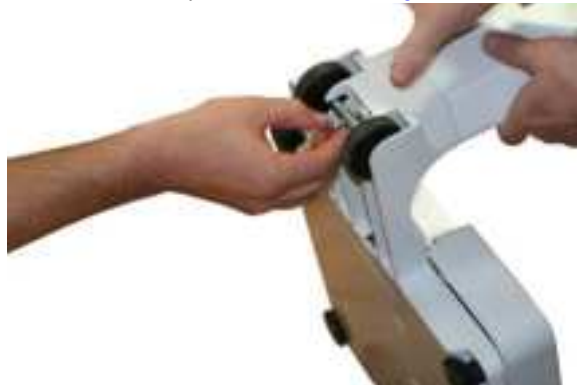
Figure 2-4. Attach Wheel Assembly
