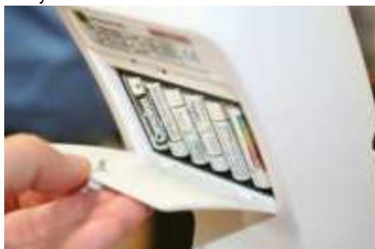
Figure 2-7. Batteries in Battery Chamber
