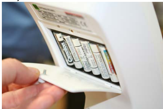
Figure 2-7. Batteries in Battery Chamber
