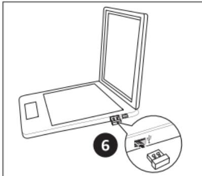
**NOTICE** The nano receiver automatically pairs with the product. If the connection fails or is interrupted, switch the product off and reconnect the nano receiver.
