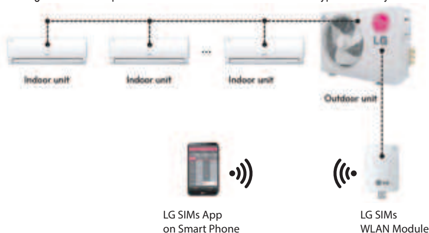
Figure 135: Example of a SIMS WLAN Module Used with a Typical DFS System.
