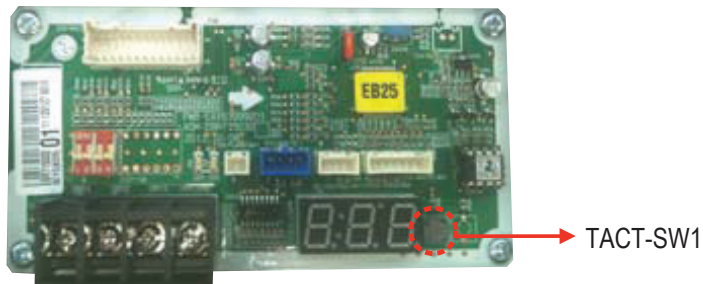
Figure 126: Location of TACT-SW1 (LMU18-24*HV).
