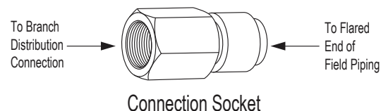
Figure 54: Connection Socket Diagram, External View.
