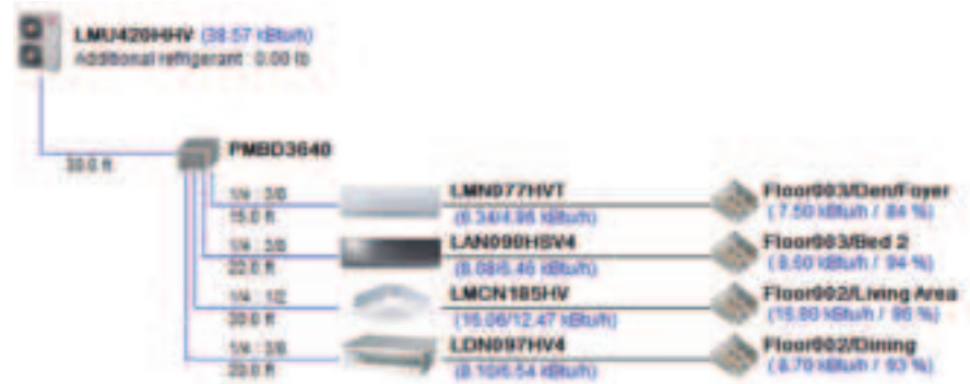
Figure 25: Example of a LATS Tree Diagram.
